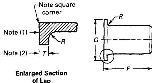
TABLE 10 DIMENSIONS OF LAP JOINT STUB ENDS
